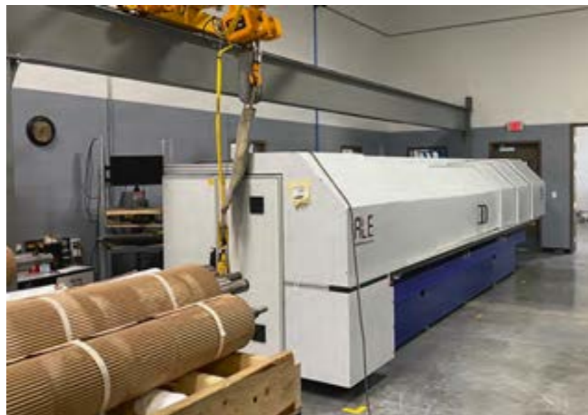
Earlier this year a new 3.5M ALE laser was installed, the third fiber optic solid state laser at the Batavia facility.
