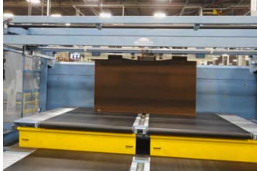
PCG added a specially designed Alliance FEEDMASTER Jumbo Bottom Feeder to the Engico's front end.
