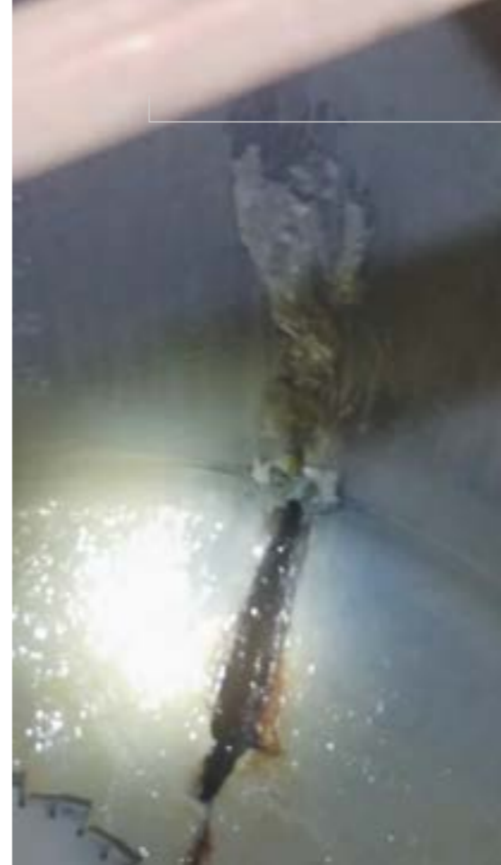
If there is a steam leak in the mixer and the lid is closed for a few hours, you will see steam inside the mixer when the lid is opened.
