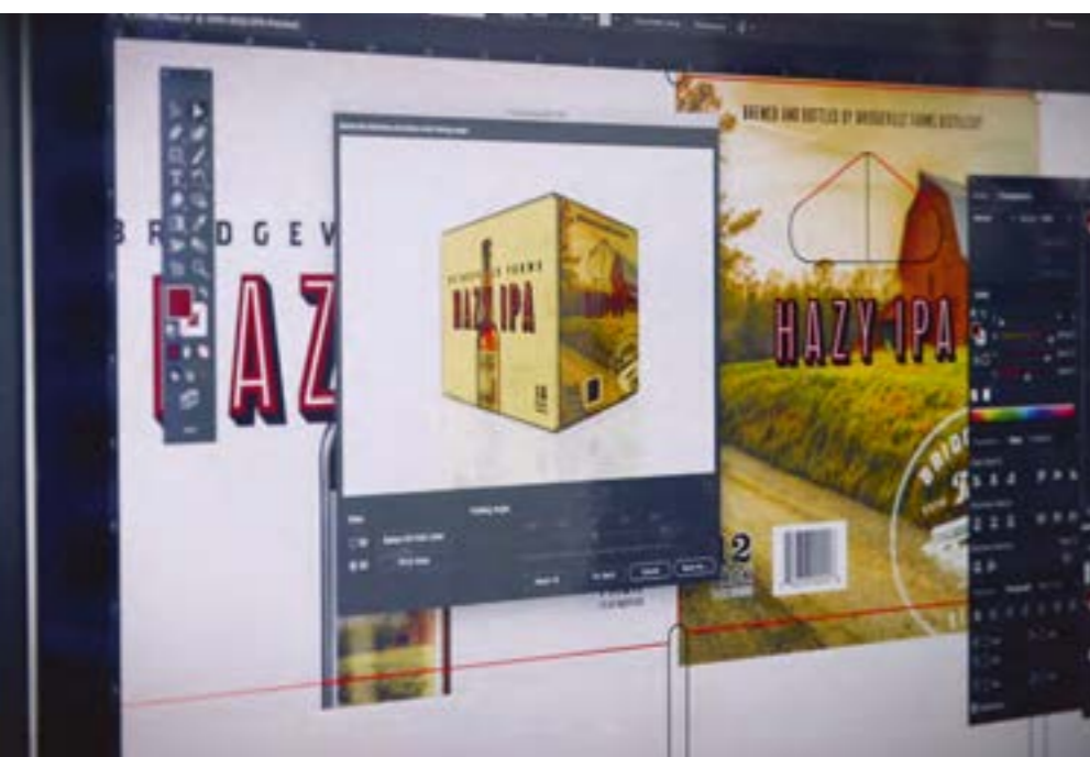
The workflow conducts all of the traditional prepress tasks like preflighting and trapping – as well as a few that are more sophisticated
