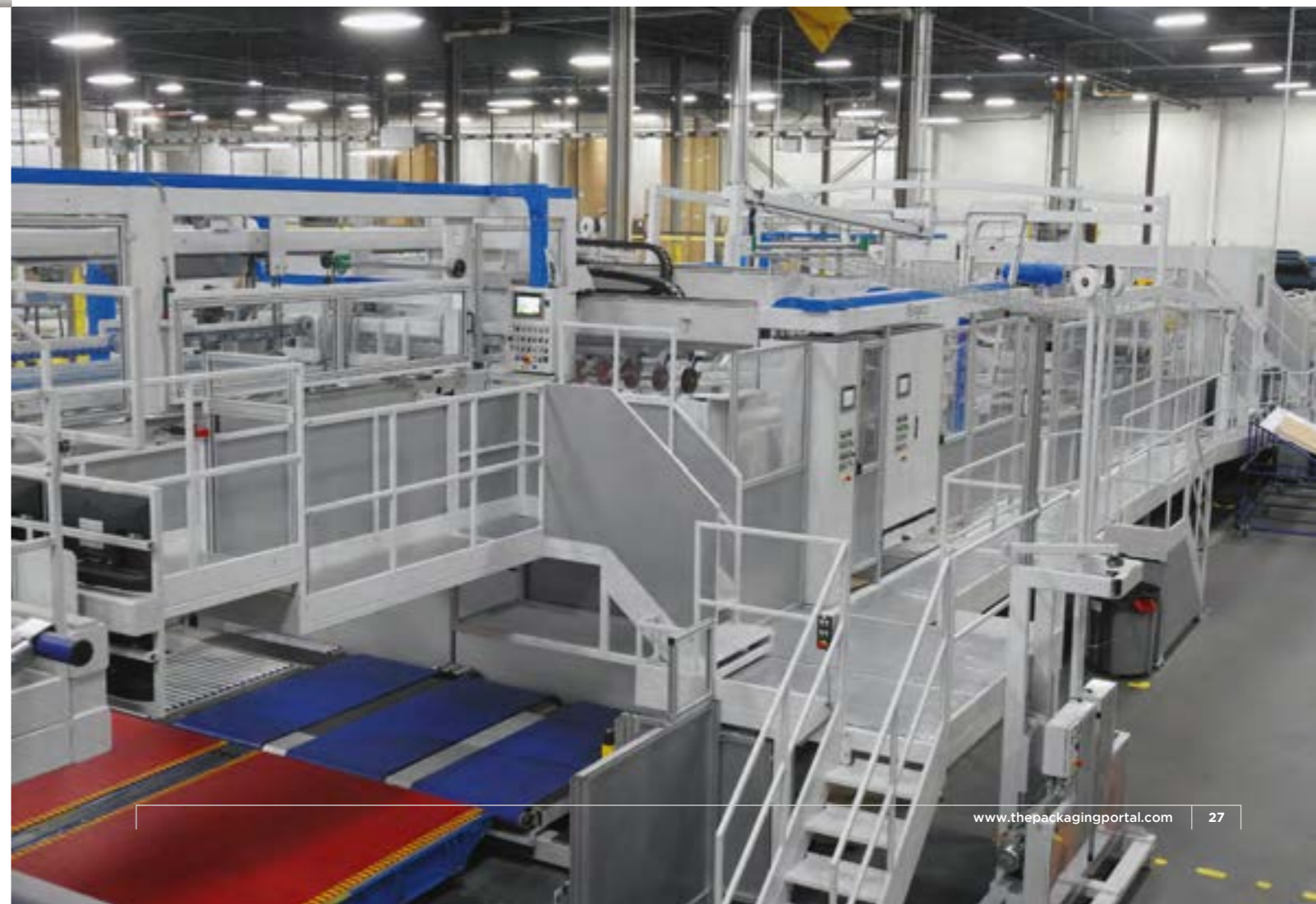
The Engico dual-sized 66/99-inch jumbo flexo-folder-gluer
