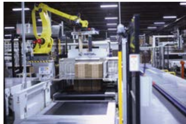
The four-color EVOL has a BW Papersystems Twin Box Slitter and an Alliance high speed top feeder and Raptor 4x2 robotic load former.
