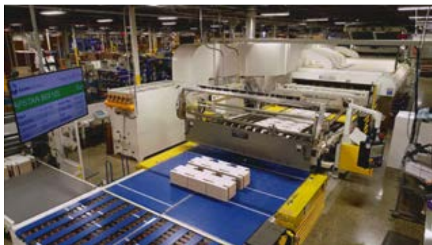
The Apstar has a Geo. M. Martin stacker and an UltraBREAK bundle breaker and UltraPAL automatic palletizer from Alliance Machine Systems International.
