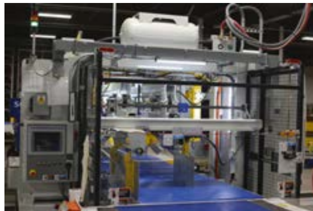
The four-color EVOL has a BW Papersystems Twin Box Slitter and an Alliance high speed top feeder and Raptor 4x2 robotic load former.
