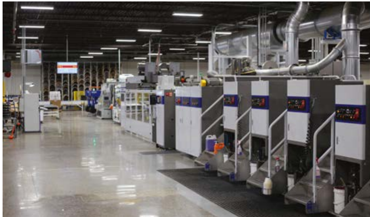
The four-color EVOL has a BW Papersystems Twin Box Slitter and an Alliance high speed top feeder and Raptor 4x2 robotic load former.
