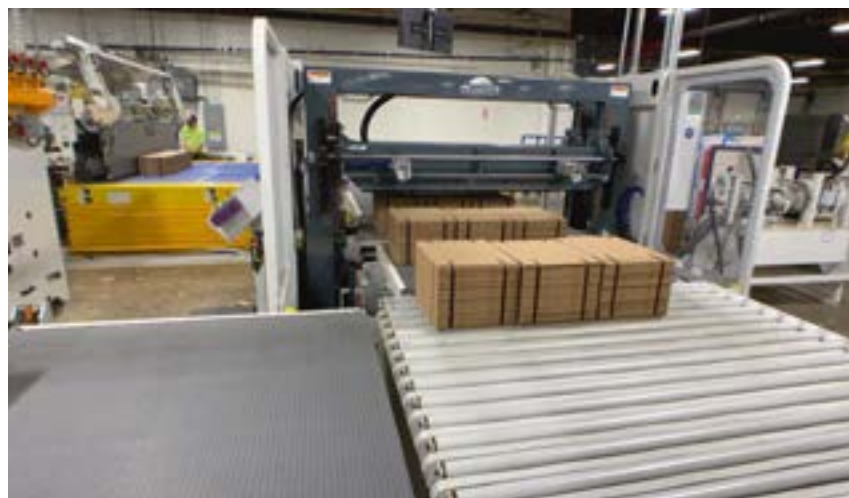
The Apstar has a Geo. M. Martin stacker and an UltraBREAK bundle breaker and UltraPAL automatic palletizer from Alliance Machine Systems International.
