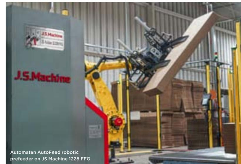
Automatän AutoFeed robotic prefeeder on JS Machine 1228 FFG
