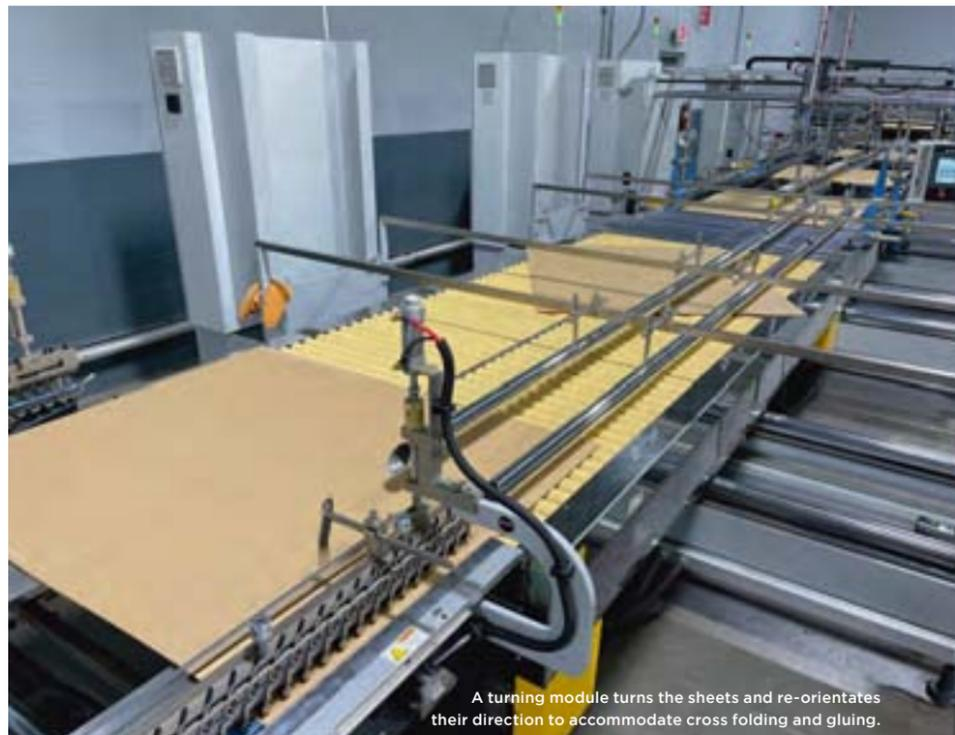
A turning module turns the sheets and re-orientates their direction to accommodate cross folding and gluing.
