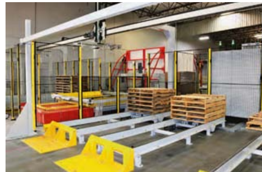
Inspire Automation's Load Pallet Device and FastPal multi-line pallet dispensing system.
