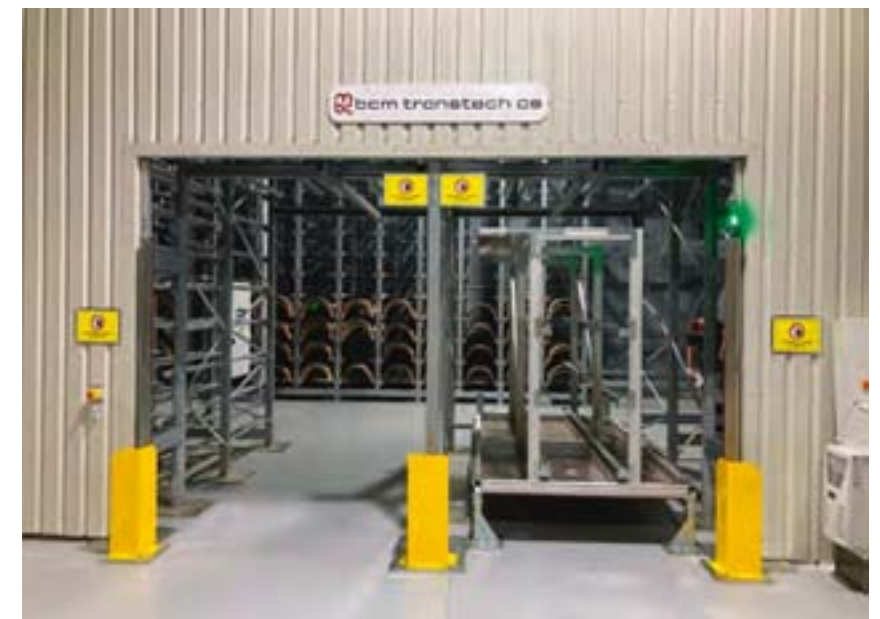
One of BCM's fully-automatic storage installations in the U.S. The storage robot will deliver rotary dies to a BCM trolley parked in a garage. An operator will pick up the trolley when the storage robot has filled it with rotary dies and drive the trolley into production.
