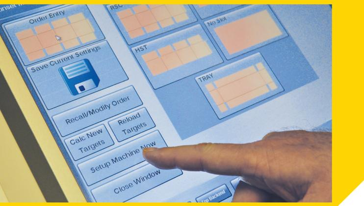
The SunSet computer control system is available as an upgrade for finishing machines and replaces obsolete systems found on Langston<sup>®</sup> machinery and other OEM's that are equipped with SUN Automation Group<sup>®</sup> products. The touchscreen operator interface allows for quick and easy machine set-up. The SunSet system stores previous order information to accurately run repeat jobs. More orders are processed per shift, reducing set-up time and waste.
