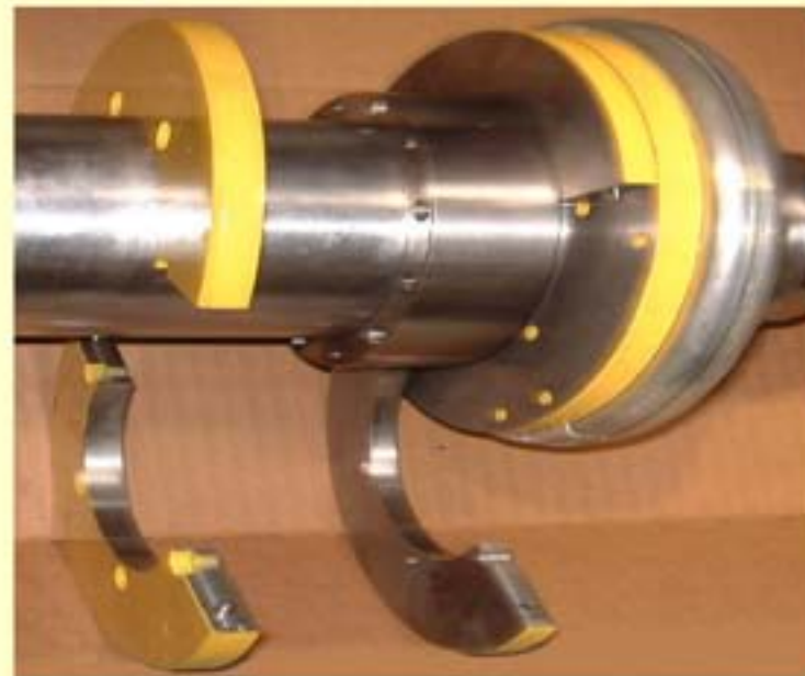
Sun Automation Group Design (only requires replacing wear plate)
